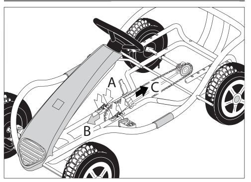
Loosen 4 screws and nuts at location A
